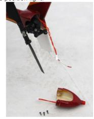
b) Remove the screws as shown from the tail frame and remove the tail frame as shown including the bearing. Disconnect the servo linkage. Then push the other bearing in the frame out of its block, only this way you can release the tail belts tension. Remove belt from pulley. Remove tail frame from tail boom by removing all three screws.
